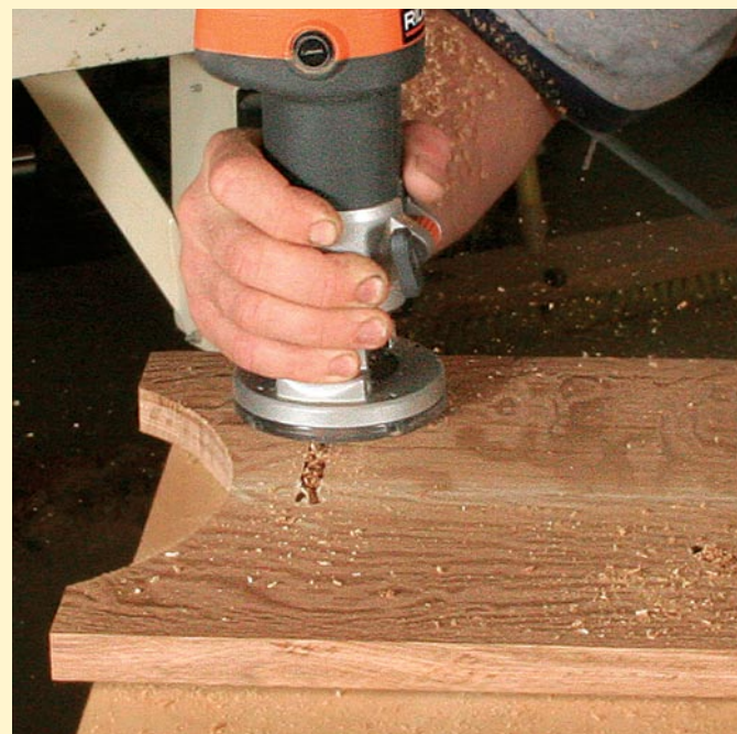
\frac{3}{8} -in.-dia. flush-trimming bit
